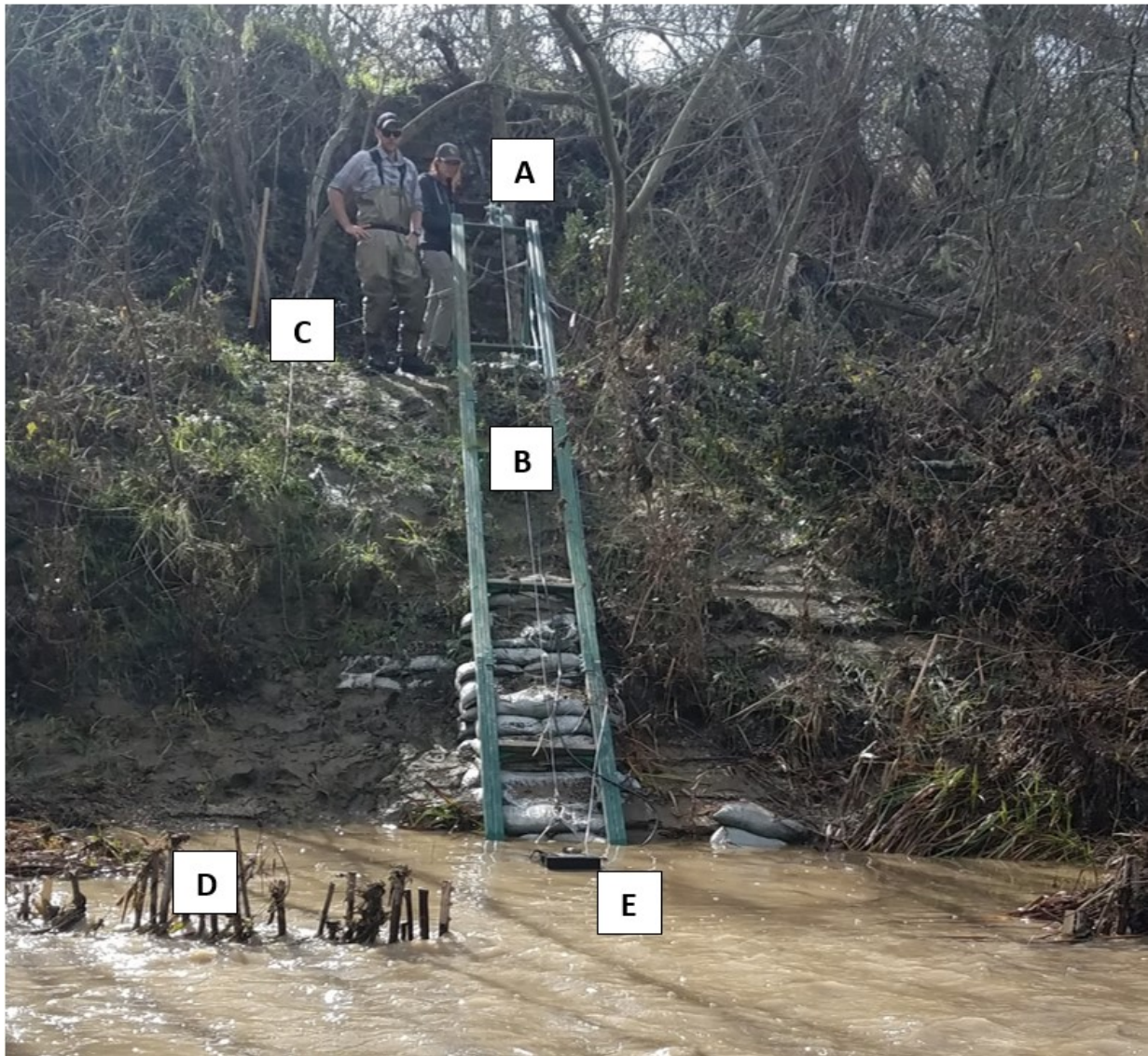
Figure 3. Salsipuedes Creek DIDSON deployment track system as seen during its last deployment in 2017 with key features labeled. (A) winch; (B) track; (C) cross-bracing cables; (D) deflection panels; (E) DIDSON/X2/sled assembly.
